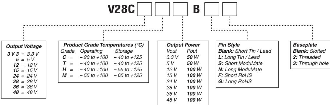
For a description of pin options, see page 9. Baseplate options include slotted flanges, threaded and through hole. See page 10 for dimensions. For other package sizes and power levels, see the Mini (half size) and Maxi (full size) data sheets.
