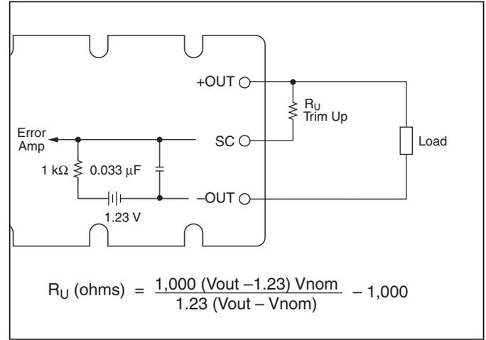
Figure 8 — Output voltage trim up circuit.
